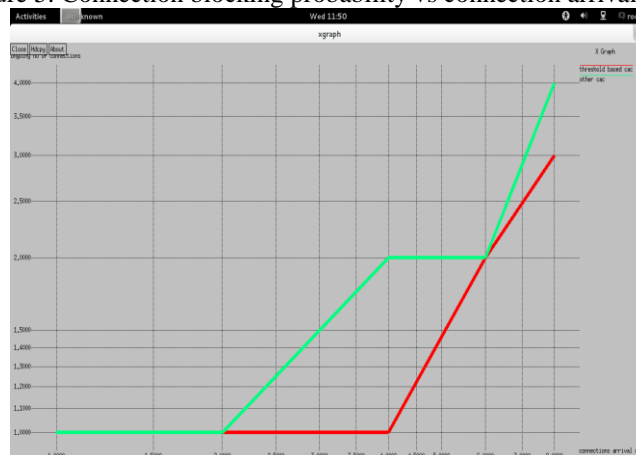
Figure 6. Connections dropping probability vs connection arrival rate.
